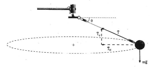
The tension in the line has been resolved into its vertical  $\overrightarrow{T}_V$  and horizontal  $\overrightarrow{T}_H$  components.
