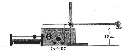
Set the rheostat so none of its resistance is included the circuit. Set the supply on 2 volt DC but do not turn it on. Check that the plastic disc on the motor shaft is horizontal and not higher than 35 cm above the level of the desk. This will ensure the ball will rotate below the eye level of a person seated.
